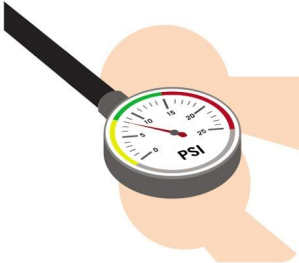
Pressurized drip system: Check pressure at the end of the drip line (8-15 PSI)
